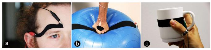
Figure 1: Polymerized tape for prototyping input devices. Here tape is used to create functional analog input on (a) the face (b) a soft, elastic object and (c) a rigid object. The elasticity and stickiness of the tape enables robust and effortless deployment, while the functional properties created by polymerization with pyrrole enable high resolution sensing.
