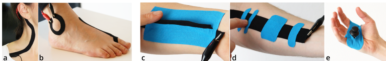
Figure 3: Kinesiography tape allows for a large variety of on-skin placements, including areas with non-uniform curvature, such as around the neck (a) or bones (b). The combination of non-resistive (blue) and pretreated (piezo-resistive, black) kinesiography tape allows using ridges and folds (c), partitions (d), and electronic components (e).
