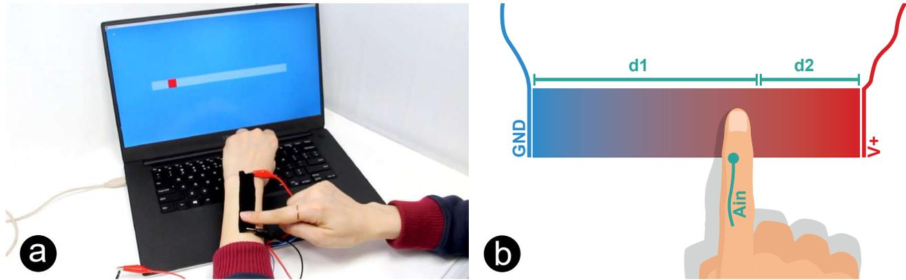
Figure 2: (a) On-Body linear position sensing and (b) the corresponding schematic. Note that the finger used for touching is instrumented to connect to an analog input where the voltage is measured.
